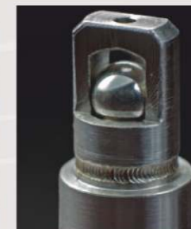
laser fine welding at a valve
