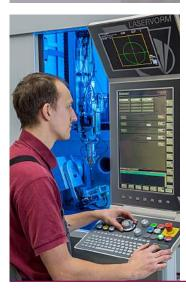
The control is the brain of the machine, it is responsible for the flawless communication between all components. LASERVORM has created a control concept which works up to 40 times faster than competitive products and which guarantees a synchronicity that is accurate to the  $\mu$  second. These characteristics allow an adaptive machining in real time.
